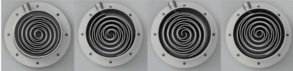
*Figure 18: Scroll movement with variable  $\theta$*
